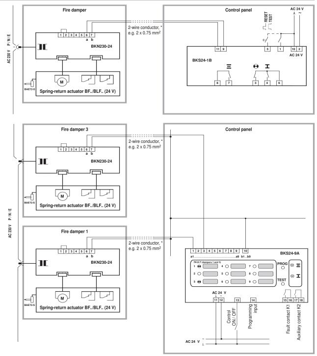
\* Lenghts of conductors: 2-wire conductors a/b max. 600 m (0.75 m<sup>2</sup>)
