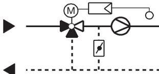
There are no restrictions with air heater mixing circuits or with injection circuits.
