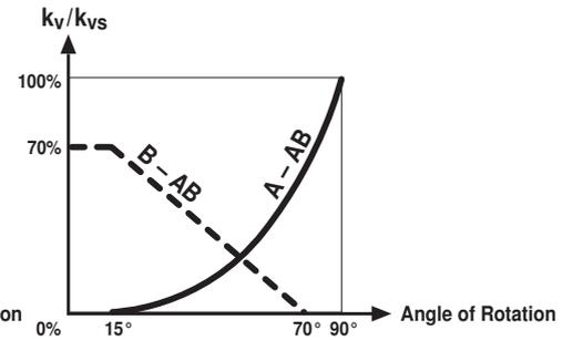
Calculation diagram for 2-way and 3-way characterised control valves R2.. / R3.. / R6..R / R7..R
