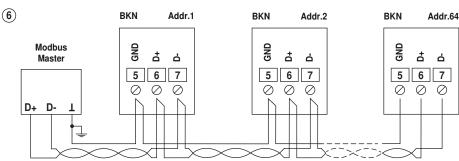
The wiring of Modbus RTU / RS485 is to be carried out in accordance with applicable regulations (www.modbus.org). The device has switchable resistors for bus termination.
