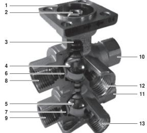
The 6-way characterised control valve was specially developed for utilisation with combined heating and cooling elements. In order to accomplish this, a 6-way characterised control valve assumes the function of four through valves or two through valves and one change-over valve.
