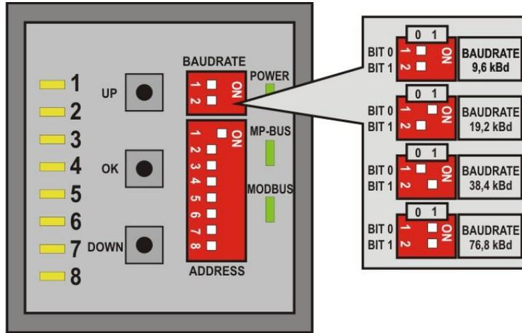
The response delay of the device is set to a fixed 4 ms with 9600 Bd. A delay of 2 ms is used as a default with higher baud rates. A longer delay can be set if needed via register 163.
