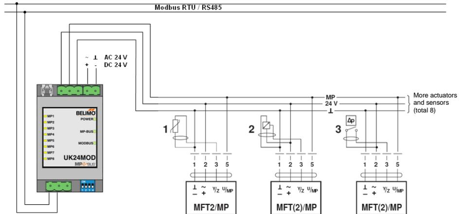
The wiring of Modbus RTU / RS485 is to be carried out in accordance with applicable directives (www.modbus.org). The device possesses resistors which can be switched on for bus connection and biasing.
