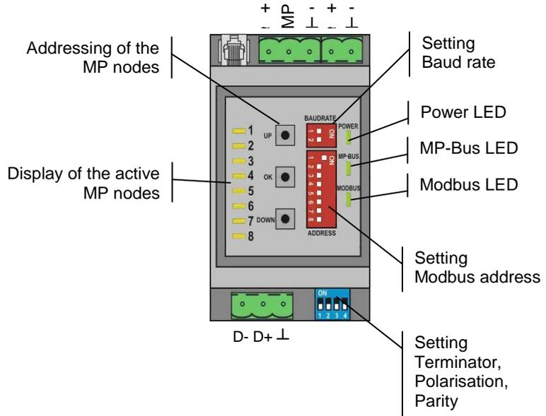
The illustration shows the operation elements of the device with the front cover open.
