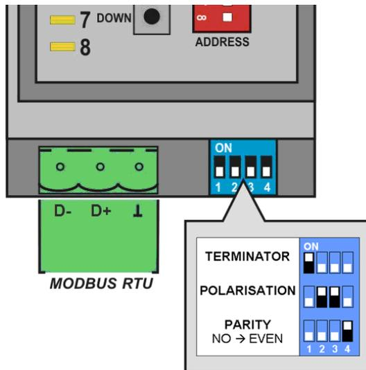
The character transmission uses either the settings NO parity (1 start bit, 8 data bits, no parity, 2 stop bits) or EVEN parity (1 start bit, 8 data bits, even parity, 1 stop bit), The setting is done with DIP switch 4.
