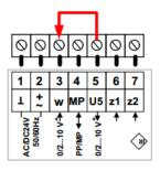
By wiring input 3 [w] of the VRP-M to the actual pressure signal [U5], it is possible to display the pressure measured by the sensor (0...10 V = 0...P'Nom) directly as a Pa value in the LON system with the open loop sensor object #1.
