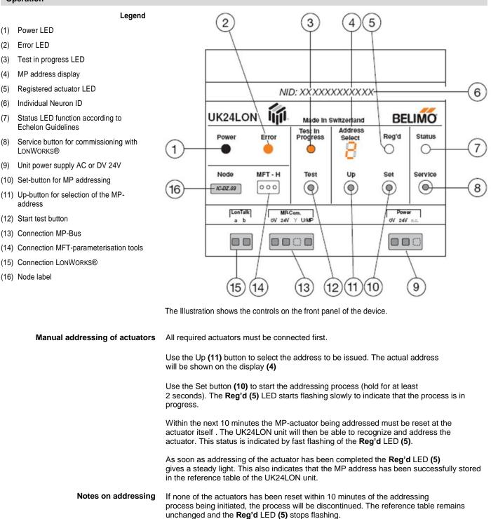
If an address is issued that has already been assigned to another actuator the latter is automatically de-addressed first before the new actuator is addressed.
